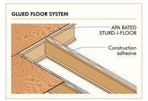
**Step 2: 1/8" Panel spacing is recommended, leaving room for expansion due to changes in moisture content.** From their initial mill-dry state, panels will expand as they reach their equilibrium moisture content. If they are installed without room to expand, panels may buckle. APA recommends leaving 1/8-inch space at all sheathing and Sturd-I-Floor edge and end joints, including tongue-and-groove joints, unless recommended otherwise by the product manufacturer.
